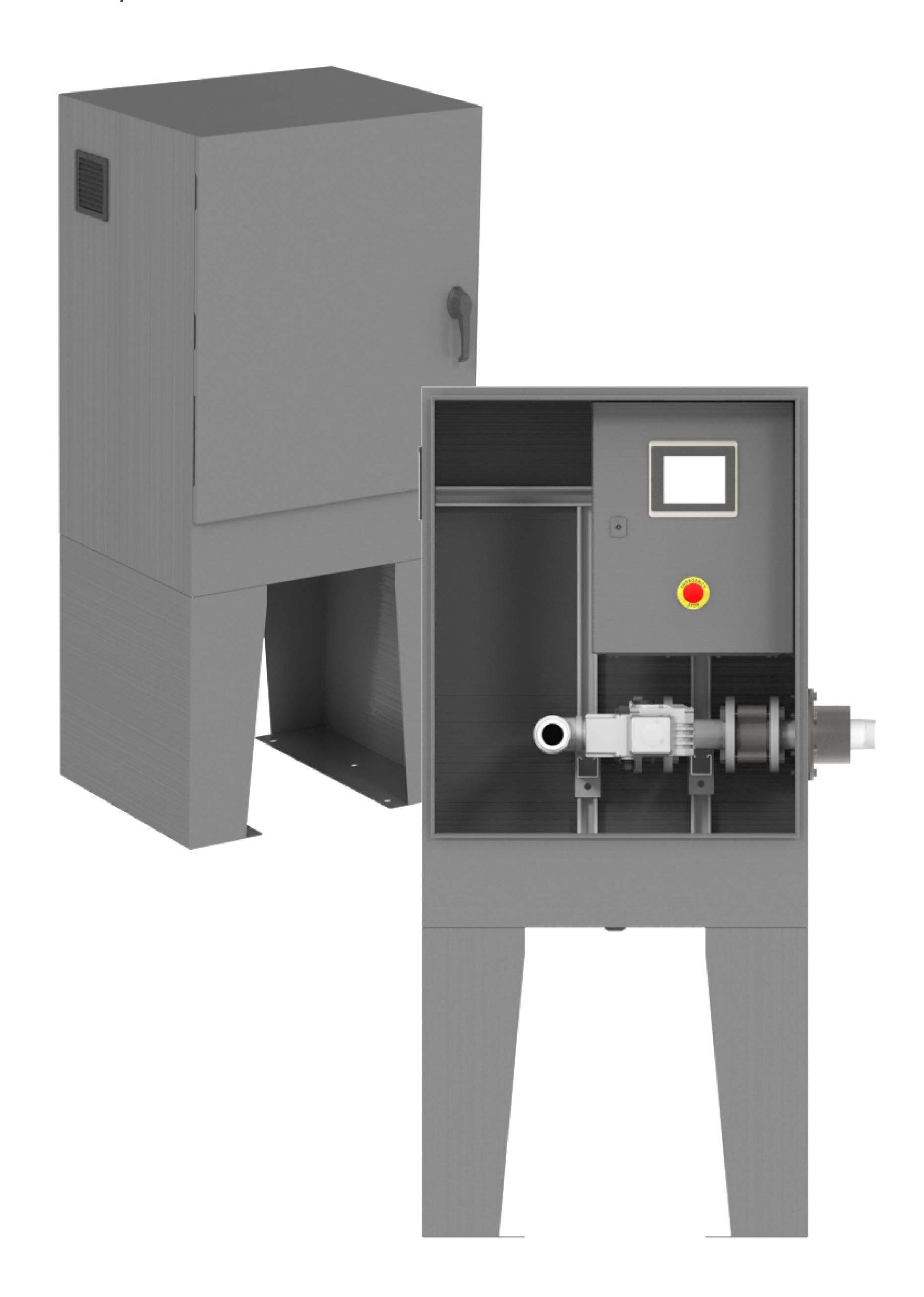
The AXI Intelligent Fill Port is capable of managing DEF distribution for multiple tanks. The System Automation Controller can manage up to four (4) fluid tanks (Smart-Comm - two (2) tanks, Net-Comm - Up to six (6) tanks). By utilizing actuated valves, the controller can distribute fluid to the appropriate tank, while monitoring respective tank levels.
